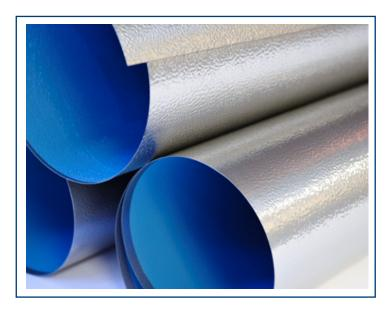
Ideal Products' Stainless Steel Jacketing with Polysurlyn Moisture Retarder is produced from T-304 and T-316 stainless steel, meeting ASTM A-240 standards. The interior of this prouct is lined with a 3 mil thick co-extruded Surlyn and Polyethylene moisture retarder. This film is laminated to the stainless steel by a process of heat and pressure. The exterior of the Polysurlyn Stainless Steel is a 2B mill finish.
